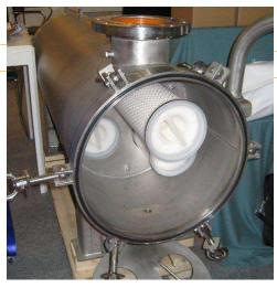
Compared with the traditional split filter element, the integrated skeleton filter element has obvious advantages. The special mechanism design makes the surface of the filter element have more uniform fluid distribution and uniform pressure everywhere, so as to improve the overall pollution holding capacity of the filter element.
