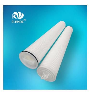
Replace EuroTec ETHF-80-40-PP-05-E filter cartridges is made from depth fine PP nonwoven fabrics. This filter has a large diameter of6 inch(152mm), single open end. The inside to outside flow pattern ensure that all the particles will be intercepted at the inside of the cartridge.
